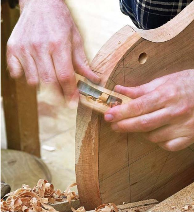
**Thumb grip.** The sole on this shave allows you to put your thumbs directly behind the blade for excellent tool control, without causing interference with the cuts.
