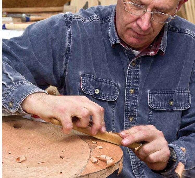
**Rapid removal.** To remove a lot of stock quickly, ride on the base of the blade with the nose of the tool up in the air. Notice my grip on the tool: My fingers are pinching in front of and behind the blade
